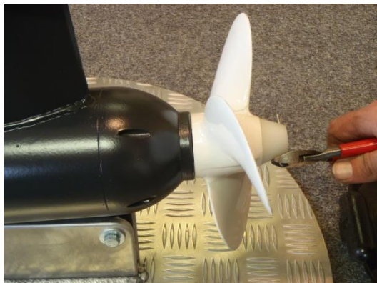
1 - Remove the cotter pin.
