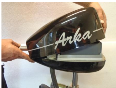
5 - Lift the hood at the back.
