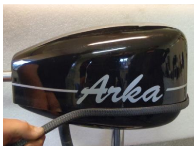
4 - Remove the rubber.
